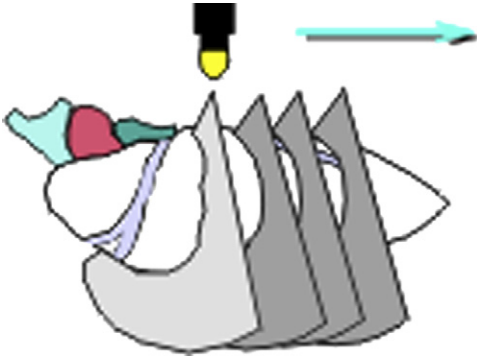
Fig. 3. Linear acquisition. Schematics of the sequential ultrasound images obtained by progressive linear, fan-like, and rotational motion of the transducer in a pre-specified fashion. Images then were reconstructed offline.
